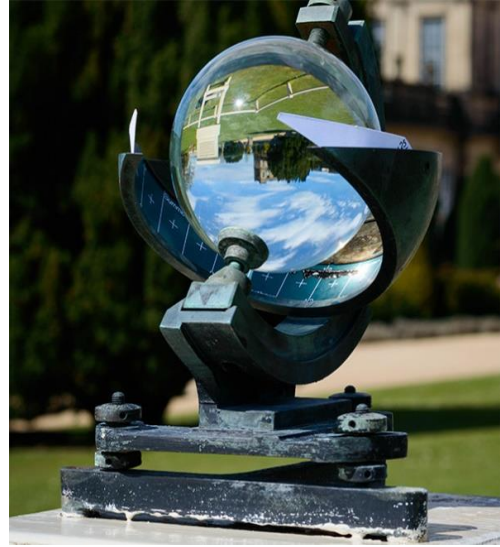
Figure 118. The Campbell Stokes sunshine recorder
